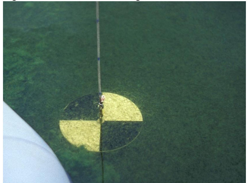
Figure 2 – Secchi Disk with floating debris in water
